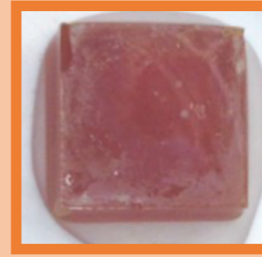
↑ GLS sample exposed to water for 10 years.
